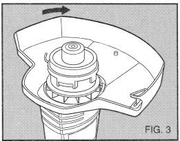
3. With the guard flanges in place, rotate the guard clockwise, as viewed in Figure 3, until it stops.
