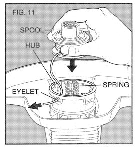
Make sure the spring is still in place in the hub. If the spool does not slip into the hub easily, press gently and pull straight out on the cutting line that protrudes through the eyelet.
