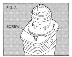
Examine the plastic guard and identify the two flanges shown in Figure 1 and the square and arrow markings.
