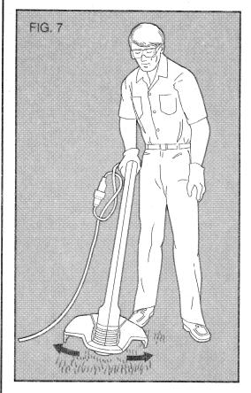
**IMPORTANT** — for the best cutting action against walls, fences and in high grass, move trimmer slowly so grass is cut **WITH THE TIP** of the high speed nylon line.
