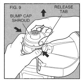
**NOTE:** It may be necessary to pull up on the shroud while depressing the release tabs one side at a time.
