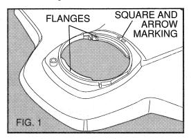
Place the guard over the spool, as shown in Figure 2, so that the square marking on the guard aligns with the the square marking on the side of the trimmer body. Place the flanges on the guard into the slots in the motor housing. Study Figures 2 & 3 carefully in order to perform this step correctly.
